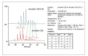
Figure 7. Analysis of cooking oil: Acclaim C30 vs. C18.
